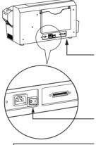
1. Place the printer in a location that allows easy access to all sides. The printer should never be operated while resting on its side or upside down.
